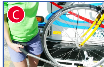
Getting Off: Raise support arm off the tire
