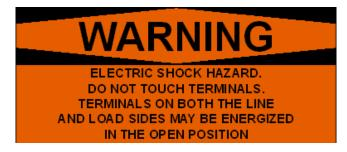
All PV system conductors shall be identified at all accessible points of termination, connection and splices. Exposed raceways, cable trays, other wiring methods, covers to enclosures of pull boxes, and conduit bodies that contain PV system DC circuit conductors shall be marked with wording: WARNING: PHOTOVOLTAIC POWER SOURCE. At the point of interconnection provide the following sign:
