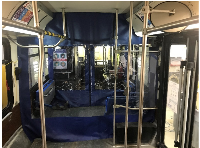
The rear plastic barrier as seen from the middle door looking toward the front of the bus. The clear plastic "window" will allow the operator to see into the passenger compartment. All ambulatory passengers will load from the rear two doors.
