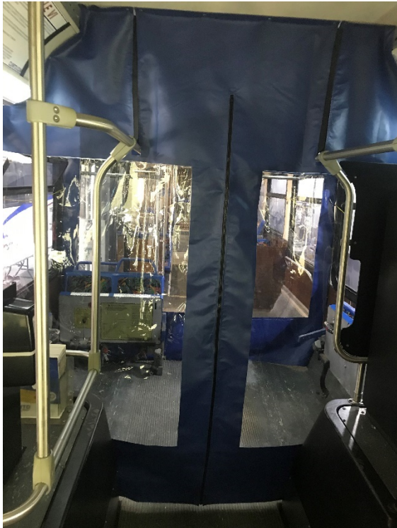
The front plastic barrier as seen from the front of the bus looking back. A zipper will make it possible for the operator to load passengers using wheelchairs into the securement area.
